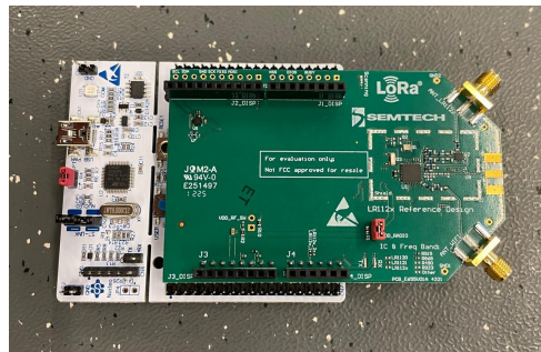
Figure 9: Semtech LR1121 transceiver with NUCLEO microprocessor board. Additionally, an antenna operating at S-Band frequency was connected to the LoRa chip, this configuration was used during laboratory tests, confirming non-degrading performance of the signal when the theoretical datasheet limit of 2.2 GHz is surpassed [46], up to 2.2005 GHz, maximum frequency selected for the mission.
