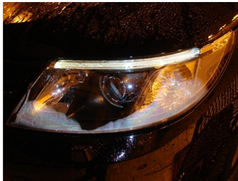
Figure 1.2: Condensation has taken place on the headlamp's outer lens [2]
